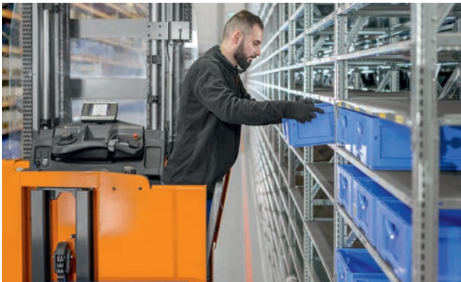
Easy access to goods no matter how far back thanks to the optional lateral tilting barriers on the operator's cab
