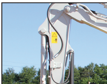
Auxiliary Hydraulic Lines
