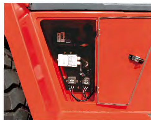
Independent integrated electric cabinet
