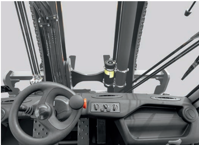
A visibility-optimised mast ensures a clear view of the goods and the working environment
