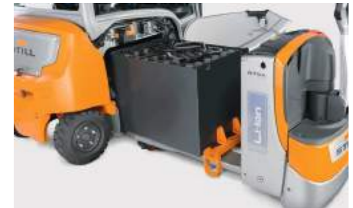
Battery change with electric pallet truck
