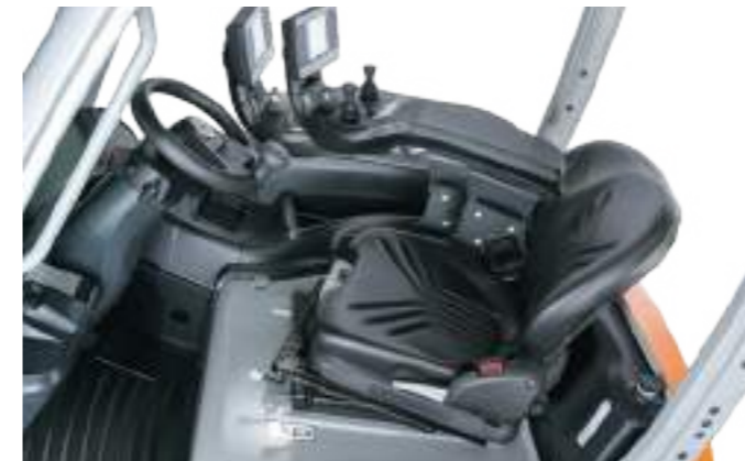
Swivel seat for comfortable reversing
