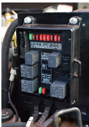
Modular high protection electrical box
