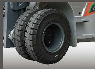
The front wheels are equipped with double tires as standard, with better carrying capacity.
