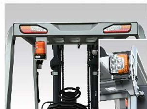
LED light of the whole truck has high brightness, long life and is more energy saving.
