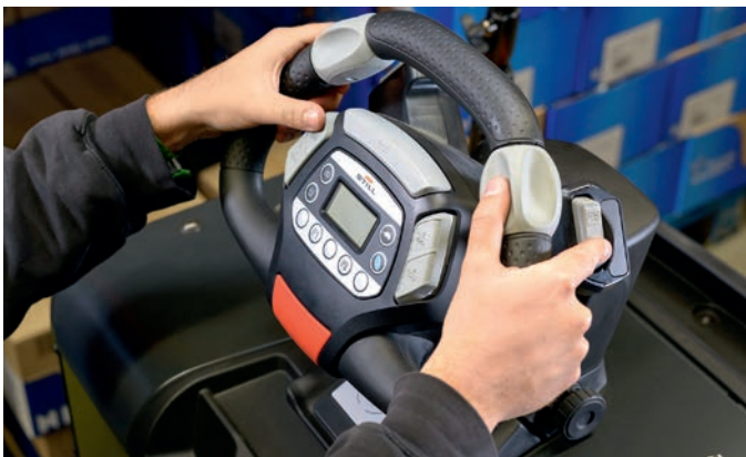
Unique STILL Easy Drive steering wheel ensures optimal driving response and allows users to operate all functions without changing hands
