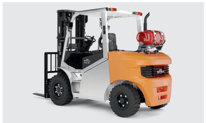
Ergonomic cylinder exchange: Hinged and swivelling holders available for different types of LPG cylinders
