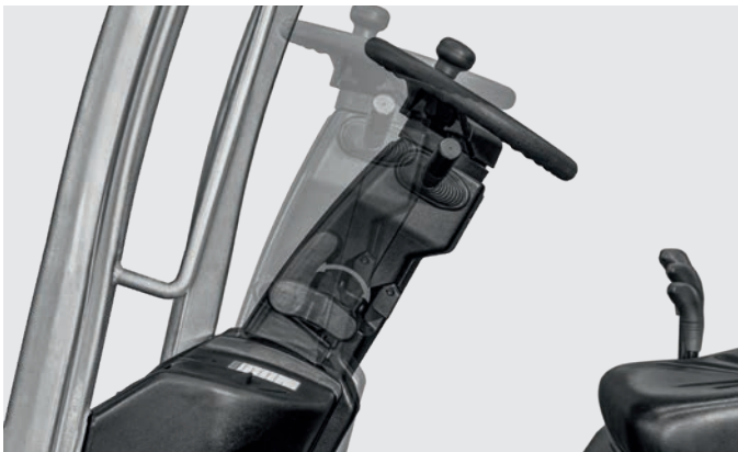
The seamlessly adjustable steering column allows operators to select the most comfortable driving position
