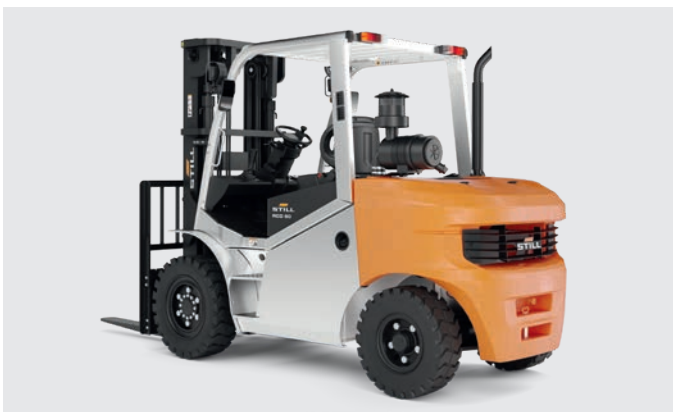
Get on and off safely thanks to the wide metal step with anti-slip profile
