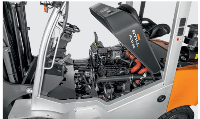
High maintainability thanks to fast and convenient access to the engine compartment**
