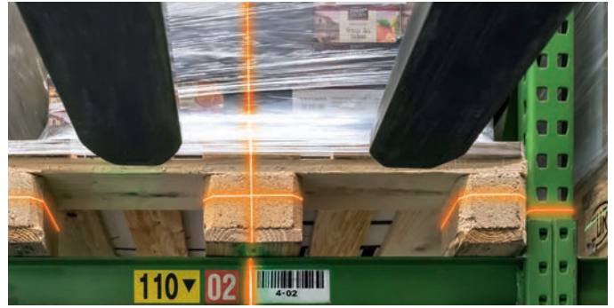
Optional cross line laser for safely aligning the centre of the pallet
