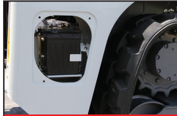
Battery Access Panel
