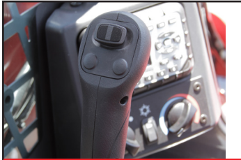
Pilot Operated Controls
