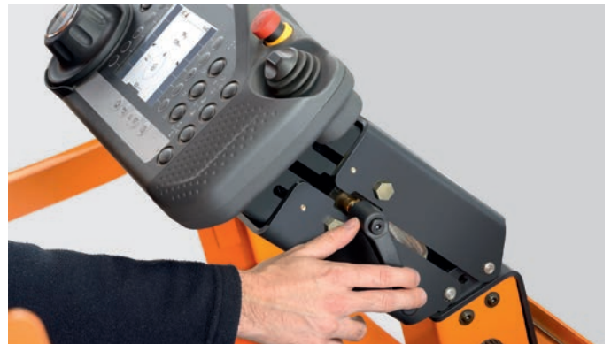
Three-dimensional positioning of the control panel
