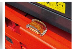
Emergency falling and dual flashing warning lights
