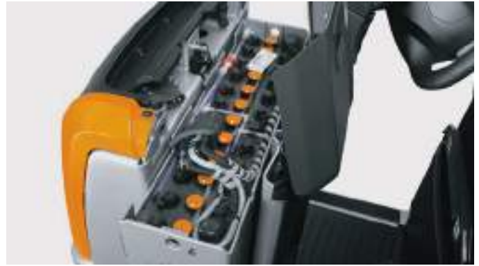
Optional lateral battery changes guarantee maximised availability and best user/driver ergonomics
