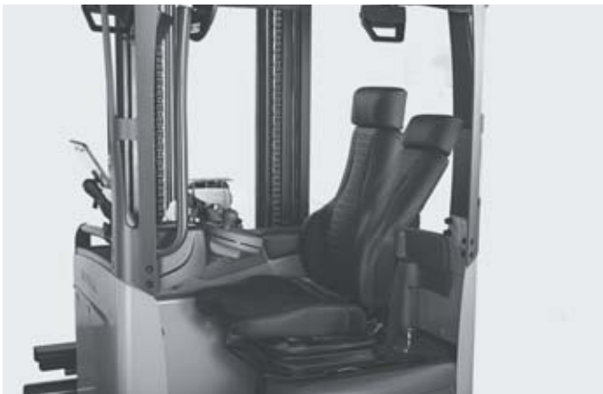
Comfortable tilt seat optimises upward visibility
