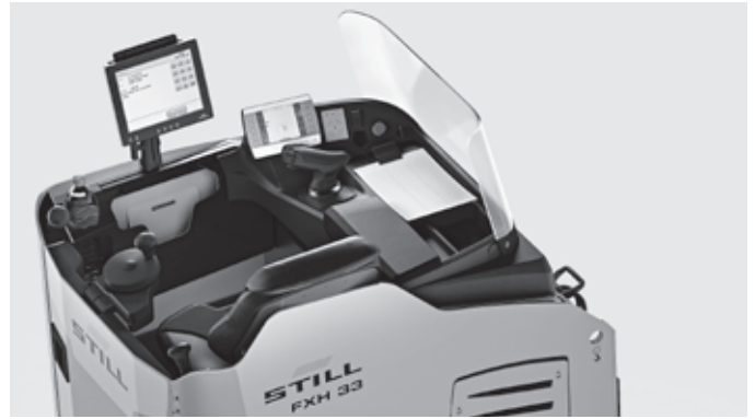
Easy positioning of optional data terminal and other accessories thanks to integrated accessory rails
