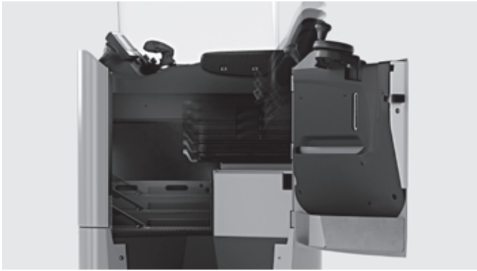
Height-adjustable foot plate that adapts to all body sizes for ergonomic working conditions
